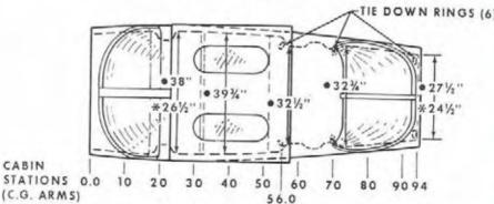
Figure 6-5. Internal Cabin Dimensions
