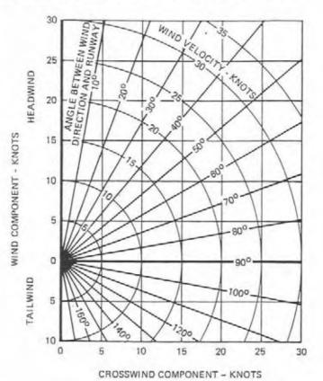
Figure 5-4. Wind Components
